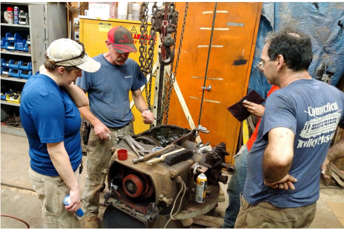
Preparing Replacement Compressor for 355
